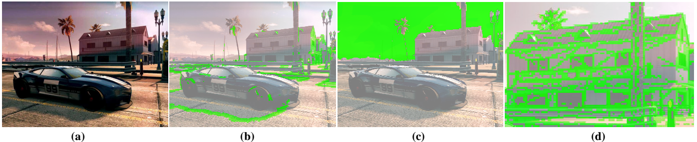
Figure 1: (a) Final rendered image, (b) Soft shadow classification, (c) Sky classification, (d) MSAA edge classification zoomed to show tile structure.
